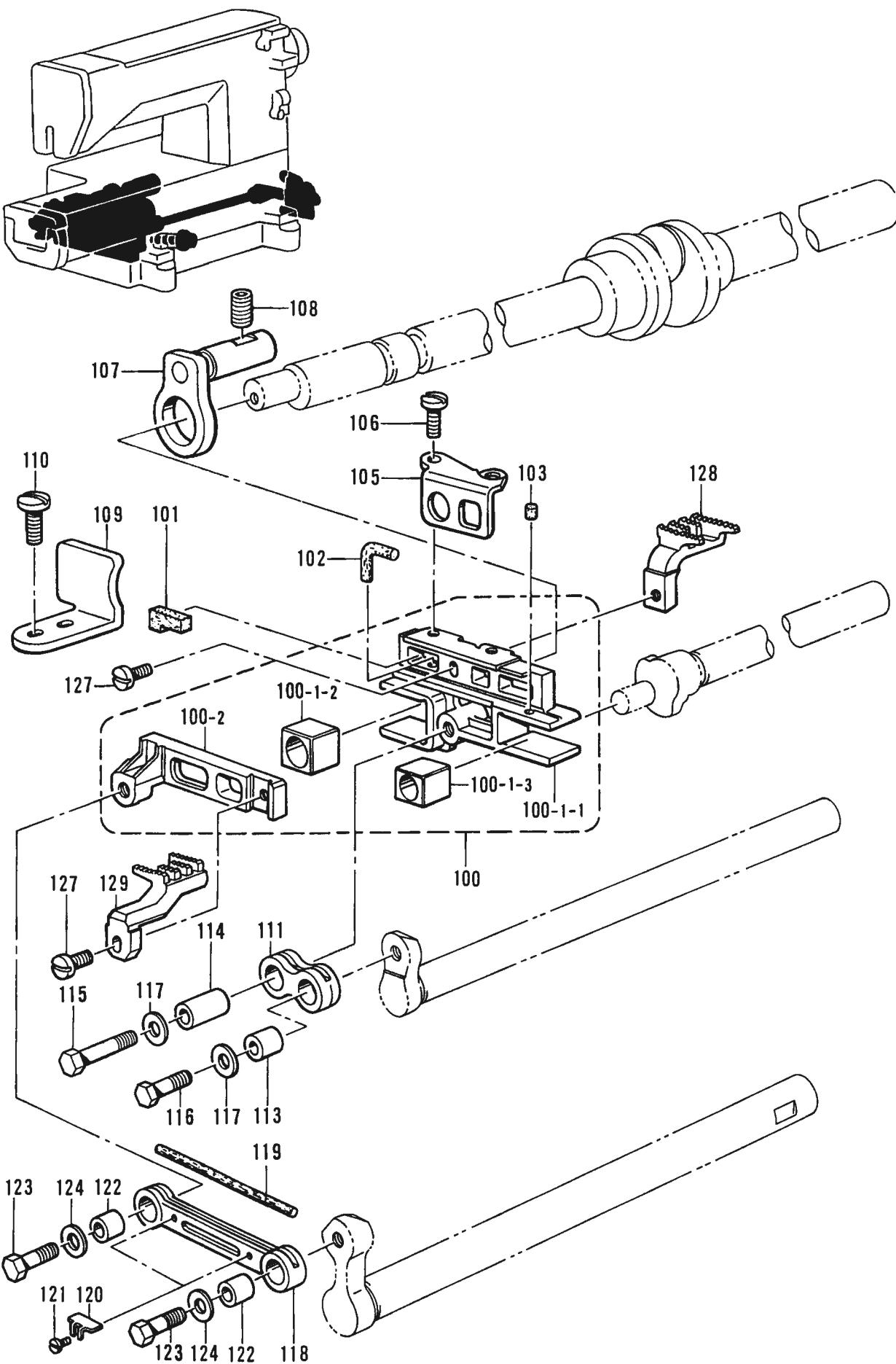
E2. 送り関係/Feed mechanism/Transportvorrichtung/
