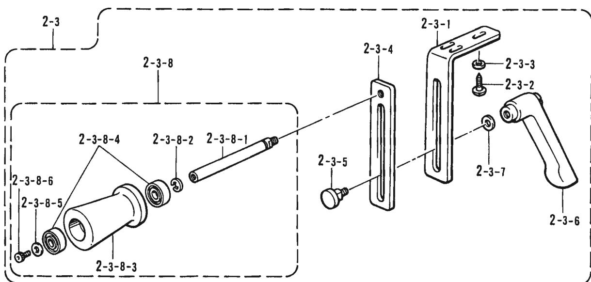
W2. 布張ローラ装置関係 / Fabric tension roller device set / Stoffspannrollervorrichtung /
