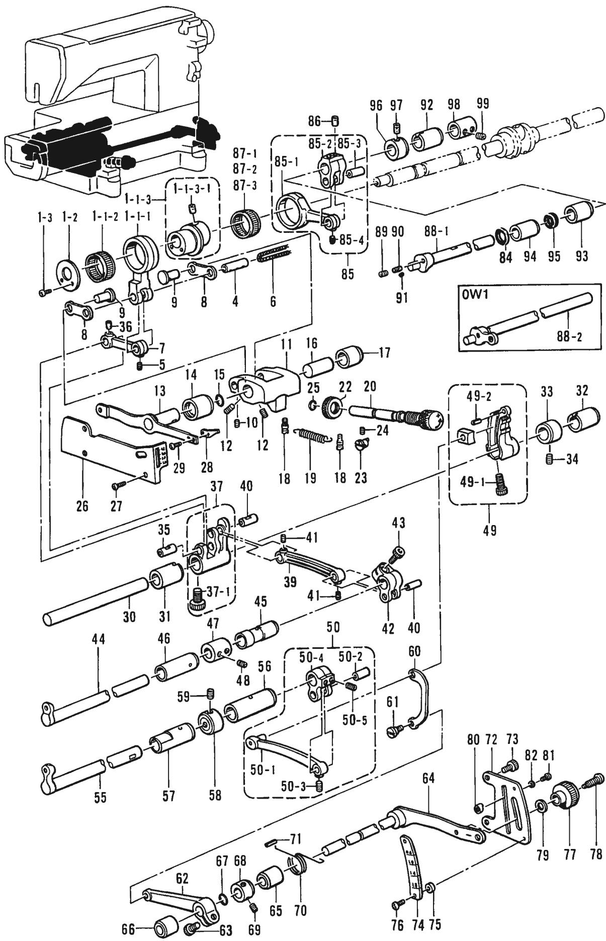
E1. 送り関係/Feed mechanism/Transportvorrichtung/
