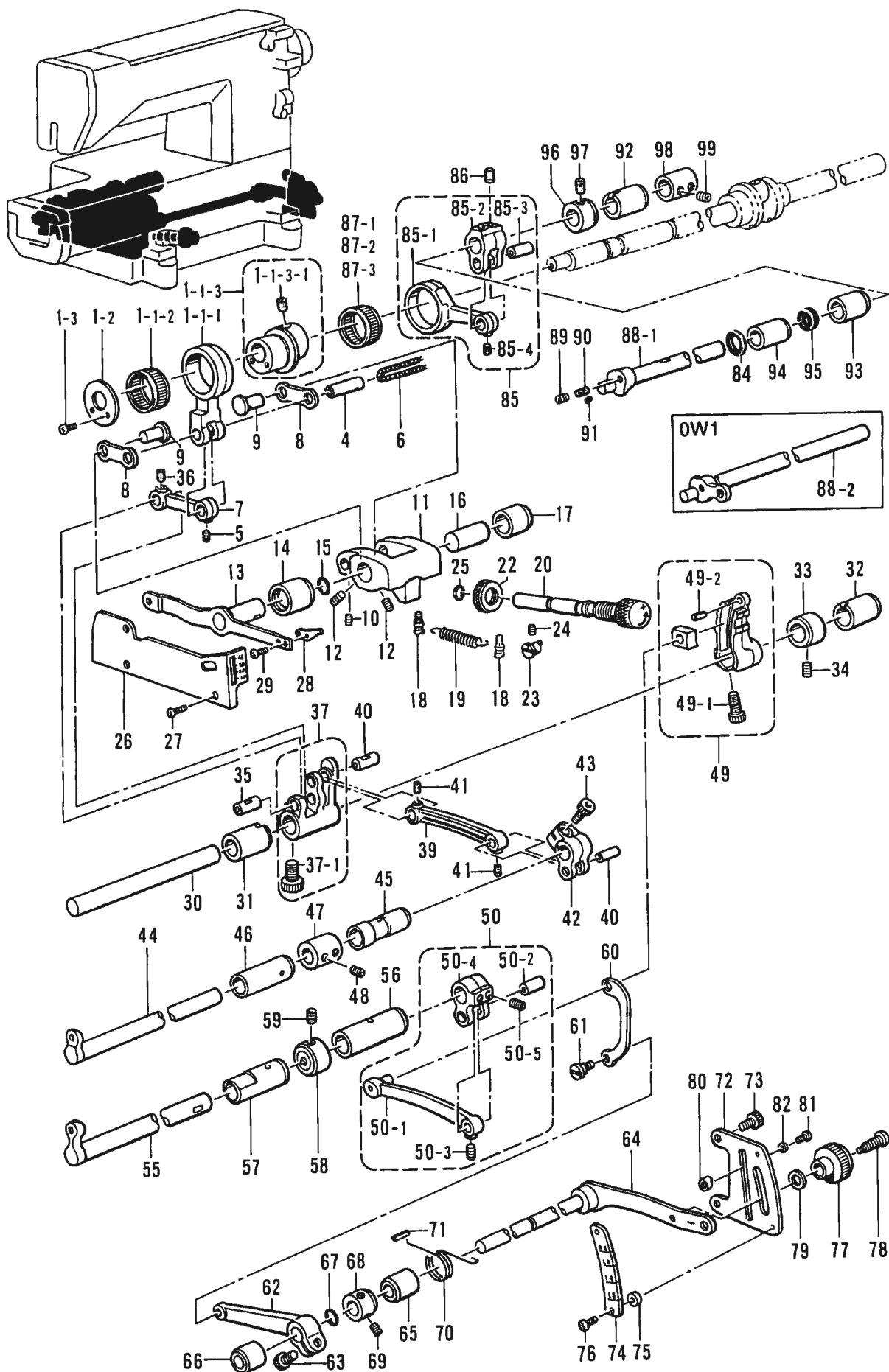
E1. 送り関係/Feed mechanism/Transportvorrichtung/
